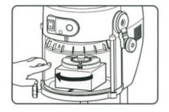
Turn the sliding cover to the left to close until the cover contacts the stopper. If it is not fully closed, the safety switch activates the unit not to work even when it is switched on.
