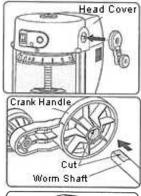
1) There is an opening on the right side of the head cover. Attach the crank handle to the body through the hole to connect the worm shaft
