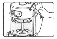
5) Turn the crank handle counter-clockwise to keep the ice holder to the lowest level. Close the sliding cover (shaving shield).
