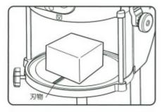
Place a block ice on the center of the shaving table. The ice should not exceed the area of the shaver blade. Otherwise ice cannot be shaved well or shaved improperly and jumps out.
