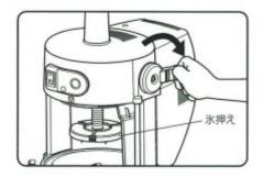
Turn the crank handle clockwise to raise the ice holder. Make sure that the ice holder does not descend when the crank handle is free from your hand. If it falls down, turn the tension bolt clockwise to hold the position so as to avoid accident.
